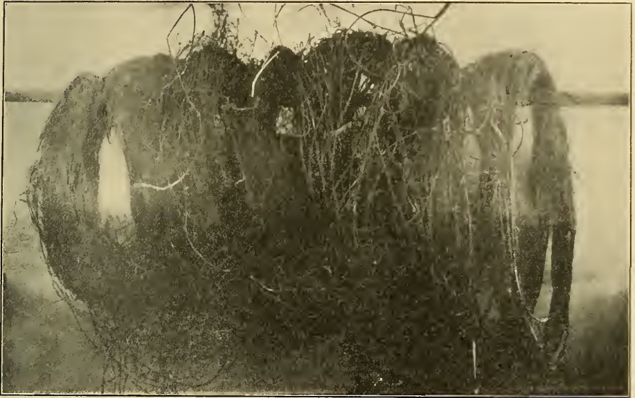
FIG. 1.—Showing pear tree root taken from drain tile.
